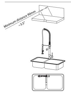
The minimum distance between the faucet hole and the wall should be 3.5"
