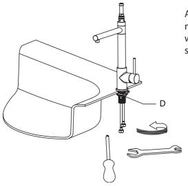
Adjust faucet body. Secure mounting hardware (D) with wrench and Phillips head screwdriver
