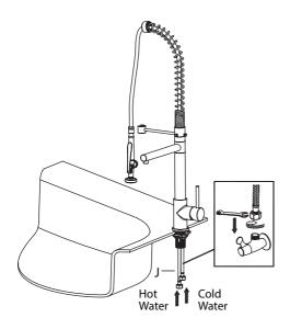
Connect and tighten waterlines (J) to angle stops. Turn on the angle stops and check for leaks (DO NOT TURN FAUCET ON)
