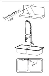
If the distance between the faucet hole and the wall is less than 3.5," position the faucet lever 30° to 90° off the wall to allow for full operation
