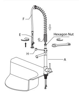
Secure spray hose (F) to faucet body (A). Insert spring (G) into sprayer holder (H). Connect spray head (E) to spray hose (F)
