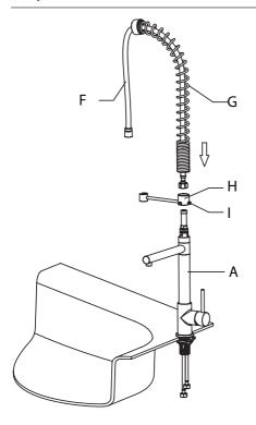
Attach sprayer holder (H) to faucet body (A). Hand-tighten thumb screws (I). Attach spray hose (F) with spring (G) attached to faucet body (A)
